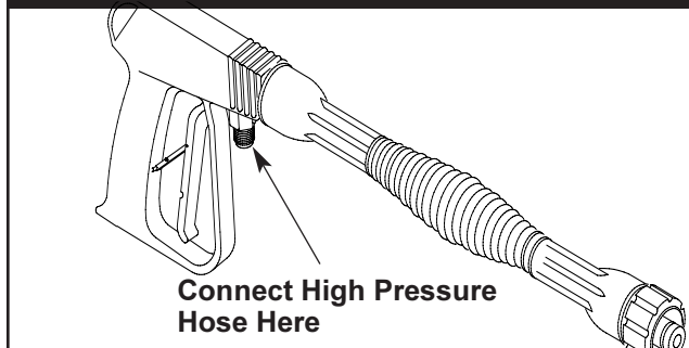
Figure 6 – Connect high pressure hose to spray gun.
